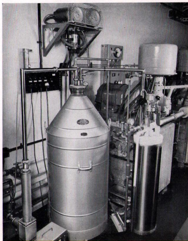
Fig. 3. Depot collector surmounted with pneumatic gun assembly, liquid air feed pipe to main reservoir liquid air feed pipe to main line assembly (with rotary pump belt guard just visible in bottom left hand corner), and wall mounted compressor to pressurize depot collector.
