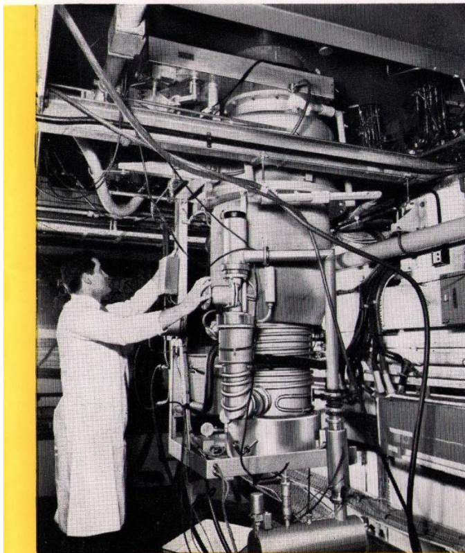
Fig. 4. 24in pumping group beneath accelerator raft showing: 24in gate valve, 24in liquid air trap, main liquid air line (top left hand), liquid air line to trap and liquid air flap valve in trap port, 24in diffusion pump and backing line.
