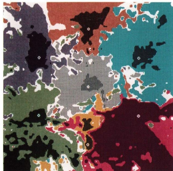
Contour plots of Carrier to Interference ratios (C/I) for a seven cell system.
